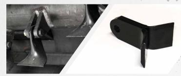
**Scoop Knife:** Used for fine or finish cutting **"Y" or Industrial Knives:** Used for tall grasses and brush
